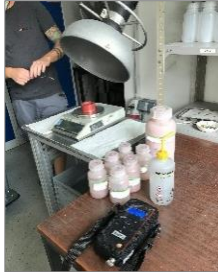
Local exhaust ventilation
